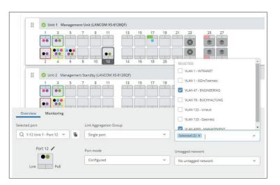
LAG setup for stackable switches
