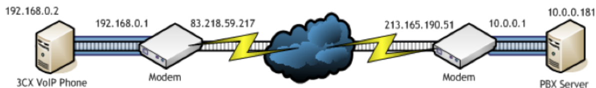
The 3CX Tunnel
